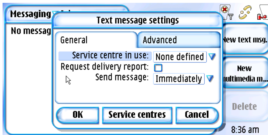
Figure 4: Calling the EditL() method on the SMS service entry brings up the SMS configuration dialog
