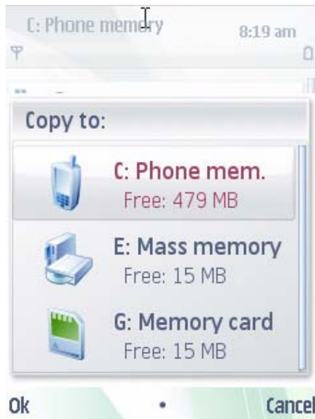
Figure 2: The Copy to: dialog showing internal mass memory and a removable memory card in addition to the phone memory
